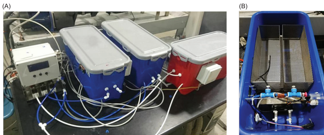
Figure 2. Pictures of the bench-top plant used in this work: (A) insulated chamber, and (B) perforated baskets.
